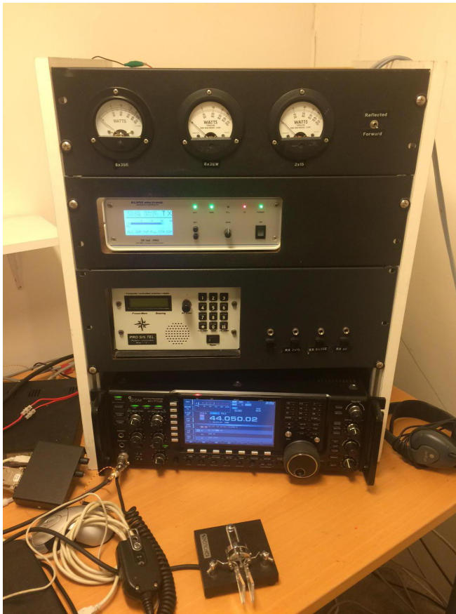
Figure 5. The transverter installed at the station.
